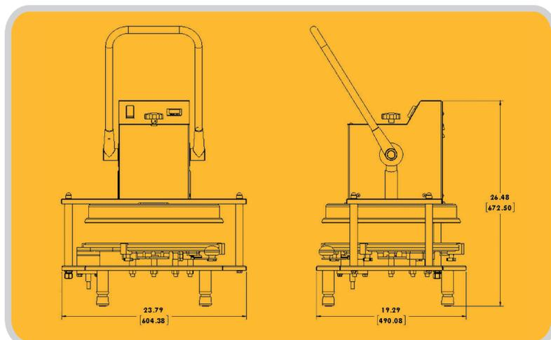
**Electrical Data:** Single Phase, 120V/60Hz or 220V/50Hz, 1600 Watts
