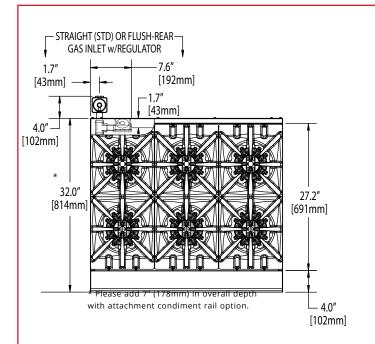
For use with Natural or Propane gas only. Gas input ratings shown for installations up to 2000 ft., (610m), above sea level. Please specify altitudes over 2000 ft. and gas type when ordering.
